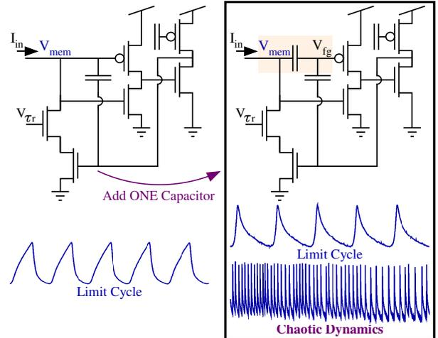
Fig. 1. Integrate-and-fire (I&F) neurons are widely employed in neuromorphic systems but generally lack complex dynamics. This work demonstrates and studies a method to instill rich dynamics, including chaotic chattering, into I&F-style neurons by altering the coupling into the gate of one transistor. This modification facilitates the parsimonious implementation of a highly nonlinear dynamical system, expanding the capabilities of I&F-style neurons.
