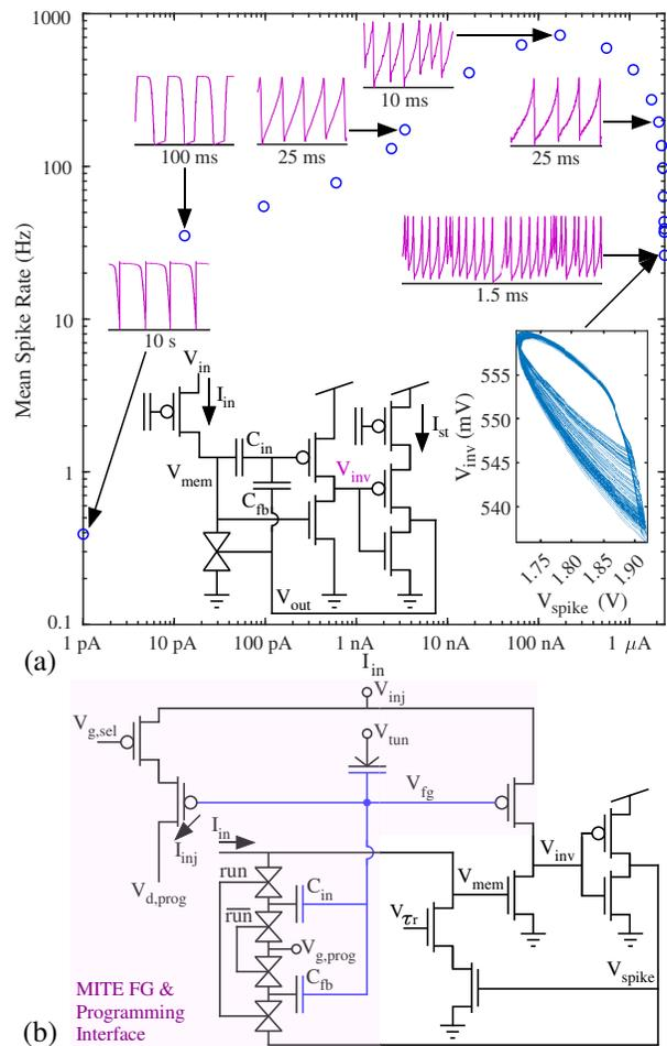
Fig. 10. (a) **Experimental** characterization of an alternative chaotic I&F neuron design using a T-gate reset mechanism and a current-starved inverter in place of a common-source amplifier, mitigating static current. This neuron exhibits an IF curve and oscillations similar to the design shown earlier, but with more pronounced bursting dynamics. (b) Conceptual chaotic neuron design for ASICs, where the  $V_{fg}$  net (dark blue) is non-contacted polysilicon.
