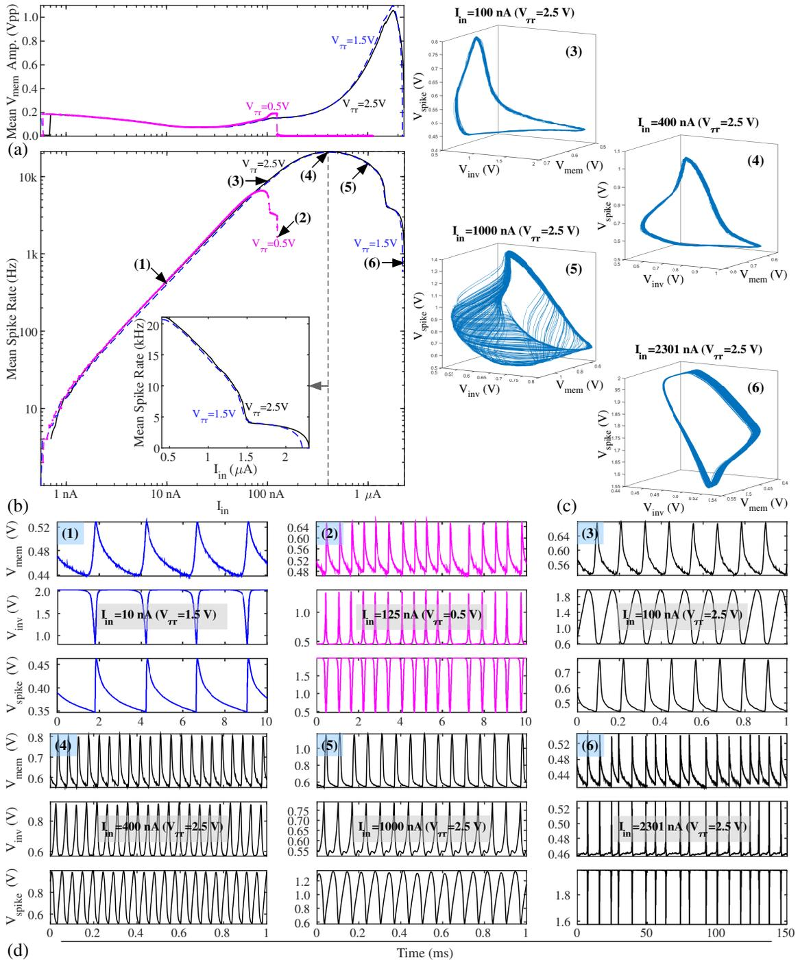
Fig. 4. Chaotic neuron **experimental** measurements. (a)  $V_{mem}$  amplitude versus  $I_{in}$ , (b) annotated IF curve, (c) exemplary attractors in the high input current regime for  $V_{tr} = 2.5$  V, and (d) nodal voltage waveforms at the exemplary spots annotated on the IF curve.  $V_{tr}$  alters the threshold current and the point along the IF curve where the response becomes nonlinear, enabling the adjustment of the mean chattering frequency and max frequency through  $V_{tr}$ .
