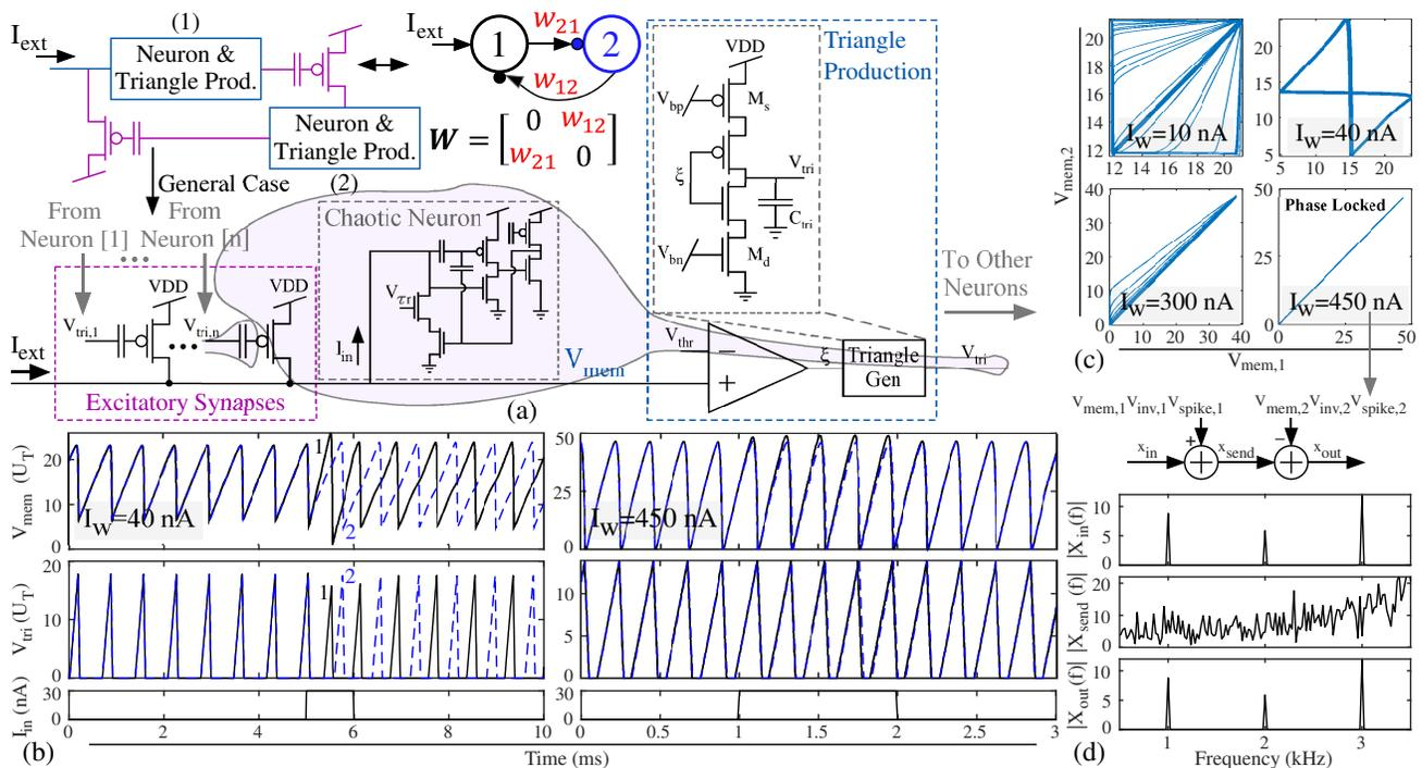
Fig. 9. **Simulations** of a chaotic two-neuron network formed by coupling our neuron model using triangle generators and FG synapses to emulate biorealistic postsynaptic currents. Network (a) signal flow, (b) response to a brief external stimulus under two synaptic weights, and (c) phase portrait after external perturbation, showing phase locking at high synaptic strengths. (d) Use of a phase-locked network ( $I_W=450$  nA) to mask and unmask a ‘secret message.’
